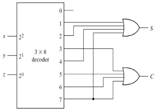
Write Verilog code to implement a full adder as given in the above circuit
